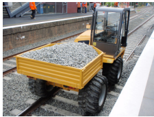
Designed for Railways work and other tight access sites: FIORI D35 JSR Dumper
