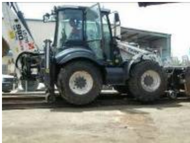
Terex 980 Elite backhoe Hi Railed for Laing O'Rourke.
