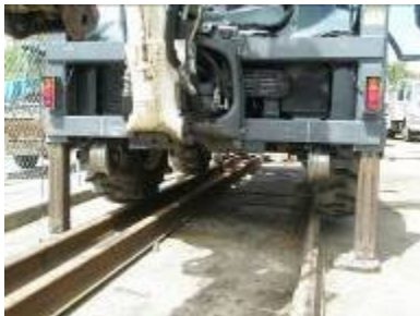
Hi-Rail adaptor fitted by to the Terex 980 Elite Melrose Mobile Hydraulics for Laing O'Rourke.
