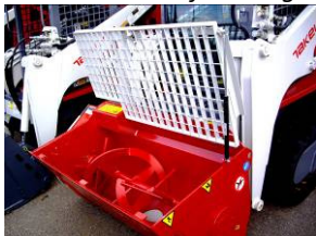
The U.Emme self-loading mini batcher/mixer makes light work of pouring pilings and footings
