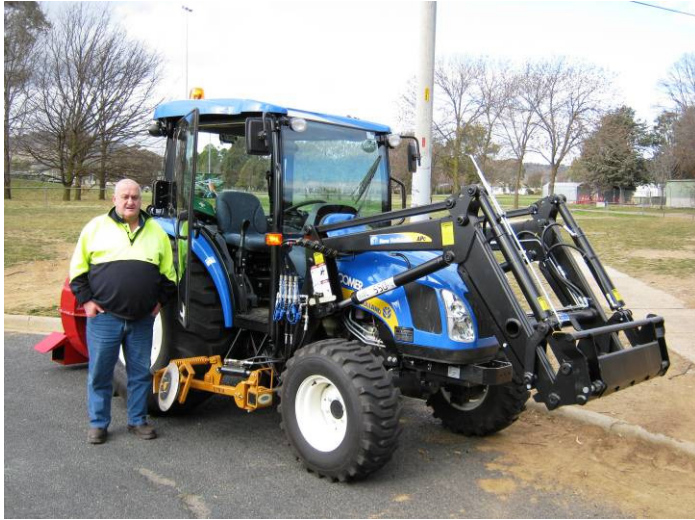
Caption: Wayne Davis, Canberra Horticulture Supervisor, with the New Holland 'Boomer' 4060 with Challenge Loader, Toro rear mounted debris blower and a mid-mount Gyral path edger.
