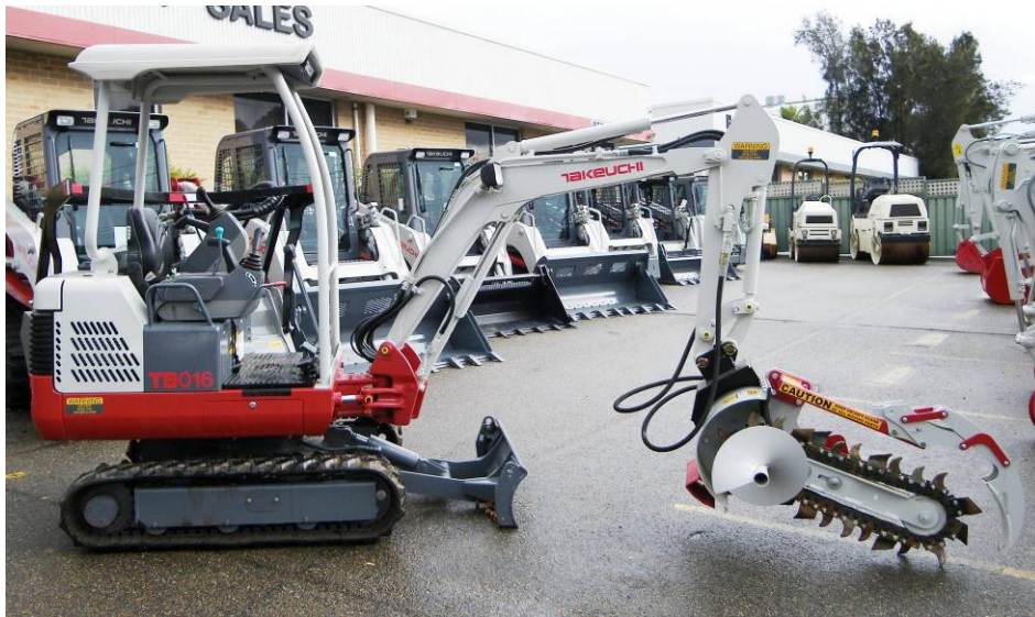
Takeuchi TB016 Excavator with the Augertorque Trencher attachment
