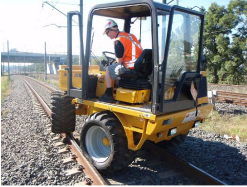
Photo: The D40 JSR's swivel steering position provides excellent control and visibility in forward or reverse.
