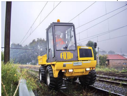
Photos: The Fiori D40 JSR Rail Maintenance Dumper: Designed to climb rails in safety.
