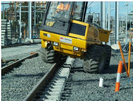
Photos: The Fiori D40 JSR Rail Maintenance Dumper: Designed to climb rails in safety.
