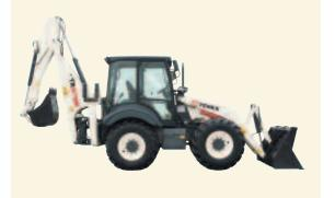
Terex loader backhoes range from 86 to 94 hp, feature operating weights from 15,151 to 17,663 lbs., and provide standard digging depths from 14 ft. 8 in. to 15 ft. 11 in.
