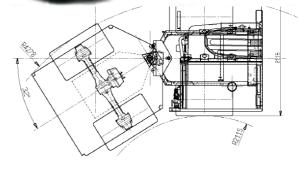
Front skip hydraulic dumping, with rear and side open able boards Max payload 4000 kg
