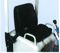
Adjustable one-piece PVC seat provides a comfortable "custom fit" for each operator, minimizing operator fatigue. One-piece PVC resists wear and tear on a tough jobsite.
