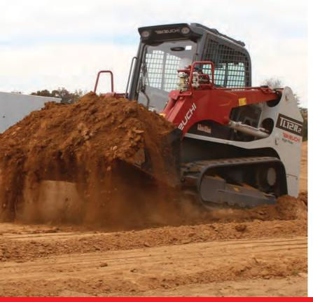
Radial arm machines feature a single arm pivot point and have higher breakout forces making them ideal for tough excavating and grading applications. They also have excellent mid-height reach which is well suited to loading and unloading flatbed trucks.
