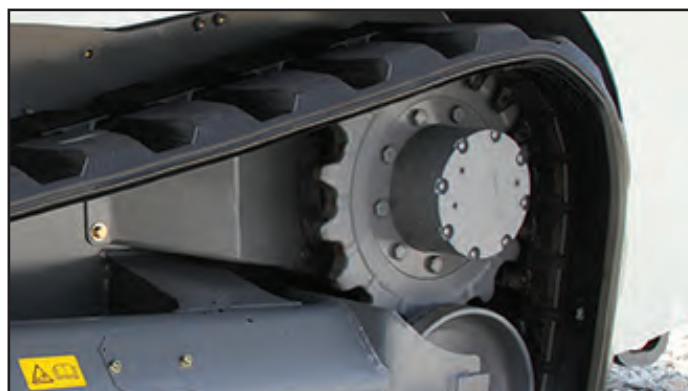
Double Reduction Planetary Track Drives
