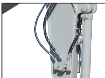
Auxiliary Hydraulic Lines
