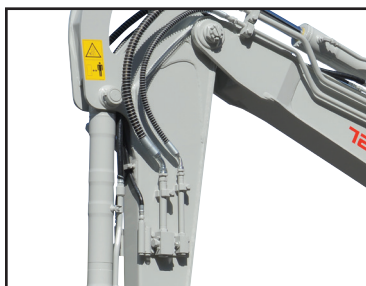
Auxiliary Hydraulic Lines
