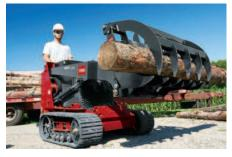
**GRAPPLE RAKE** (MODEL 22577) Grab, drag, lift and place brush and debris easily with up to 3,000 lbs (1,361 kg) of clamping force at the tine tips.
